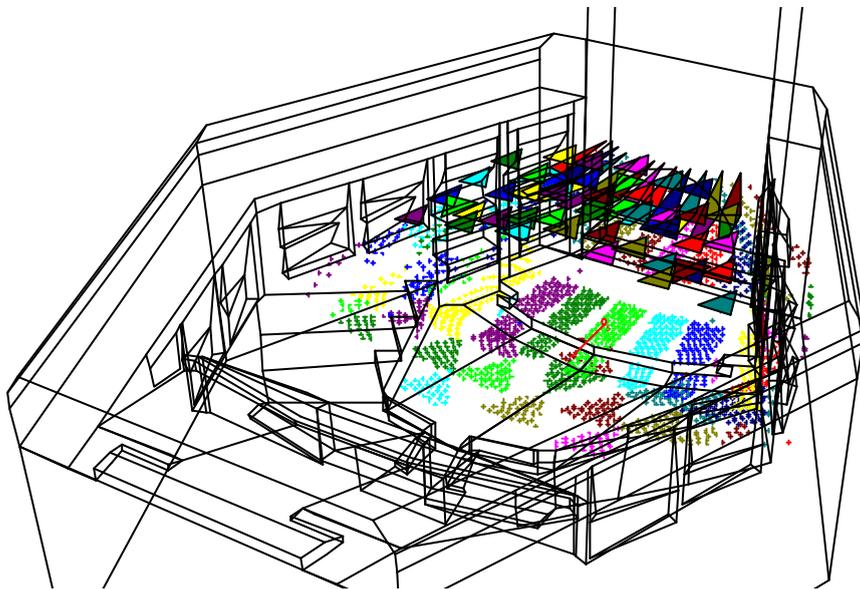
**Fig. 3** Coverage by reflectors *after* alterations.
