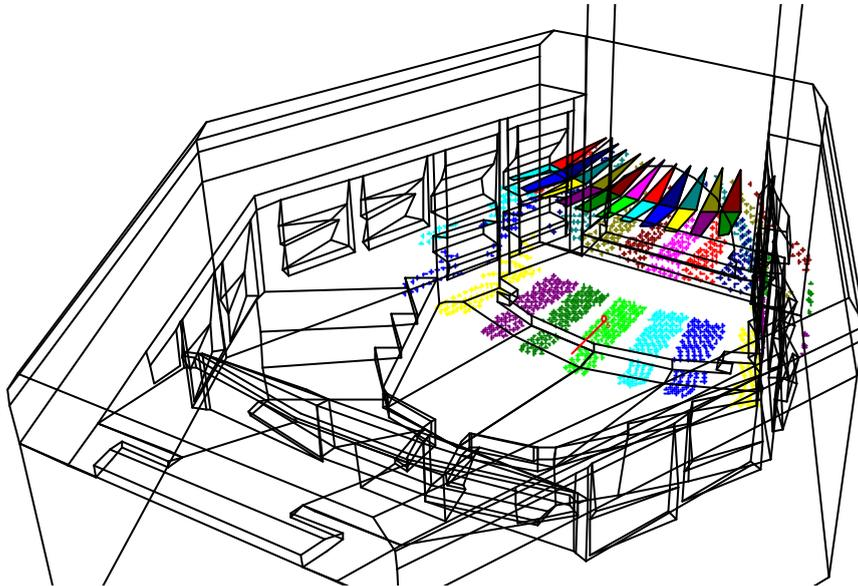
**Fig. 2** Coverage by reflectors *before* alterations.
