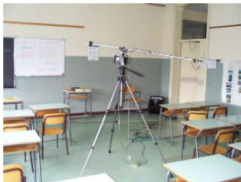
Figure 5: Pre-modification examination – in situ control of the acoustic performances.
