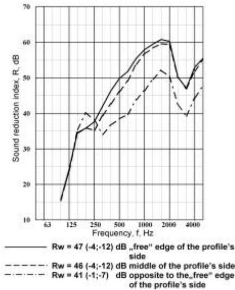
Figure 11: “Screw Position Effect” in dependence on the horizontal screw position
