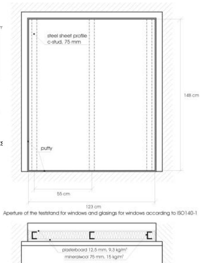
Figure 6: Situation in the test opening of the test facility for windows
