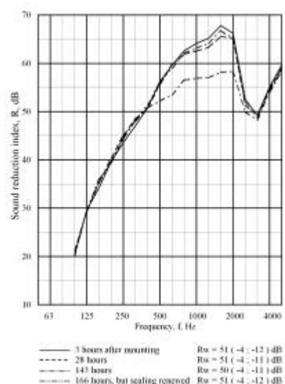
Figure 4: Effect of "ageing" of the sealant material (acrylic)
