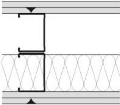
Figure 15: Section through the double-stud wall system
