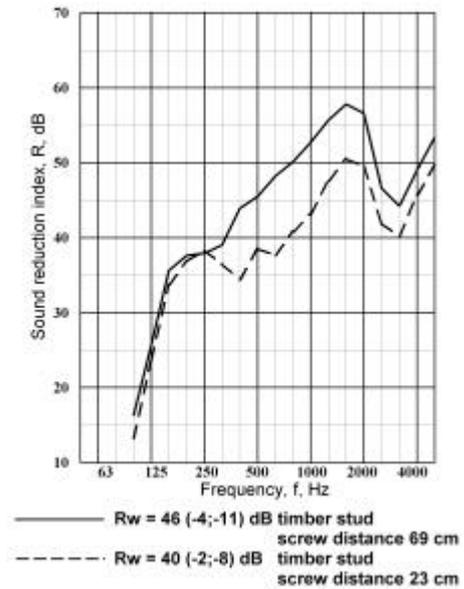
Figure 12: Influence caused by the fixing screws of plasterboard wall elements with timber studs
