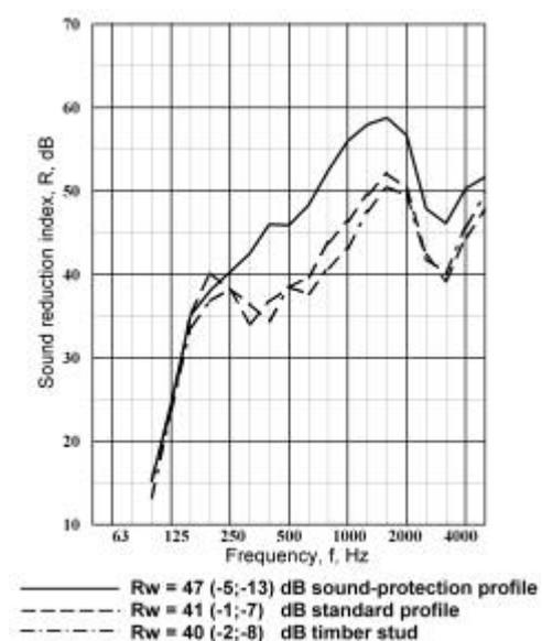
Figure 10: „Screw Position Effect“ in dependence on the kind of stud
