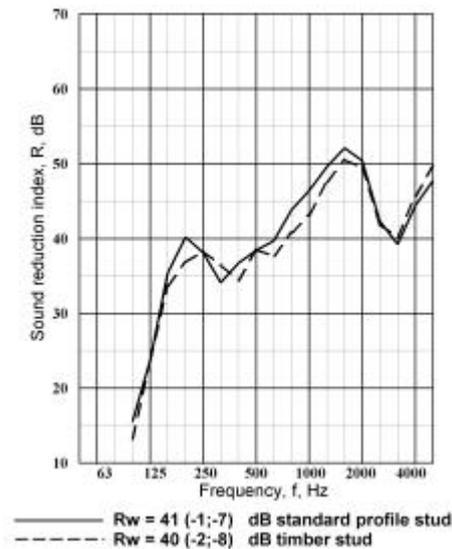
Figure 13: „Screw Position Effect“, vertical screw distance 23 cm
