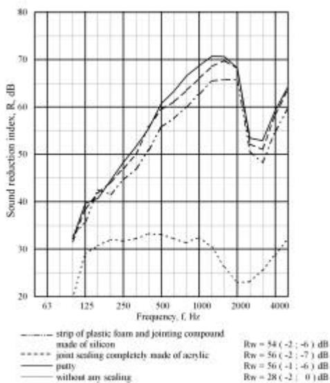
Figure 3: Influence of sealing material and workmanship
