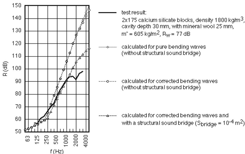
Fig. 2: Measured and calculated sound reductions indexes for a heavy double wall
