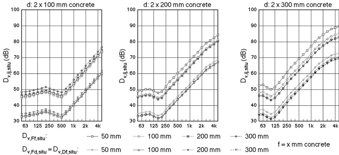
**Fig. 3:** Direction-averaged junction velocity level differences for flanking paths Ff, Fd and Df for 3 types of separating heavy double walls ( $d$ ) and for 4 types of flanking elements ( $f$ ) each.
