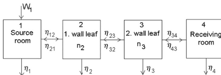
Fig. 1: SEA-systems with energy flows for modelling a double wall
