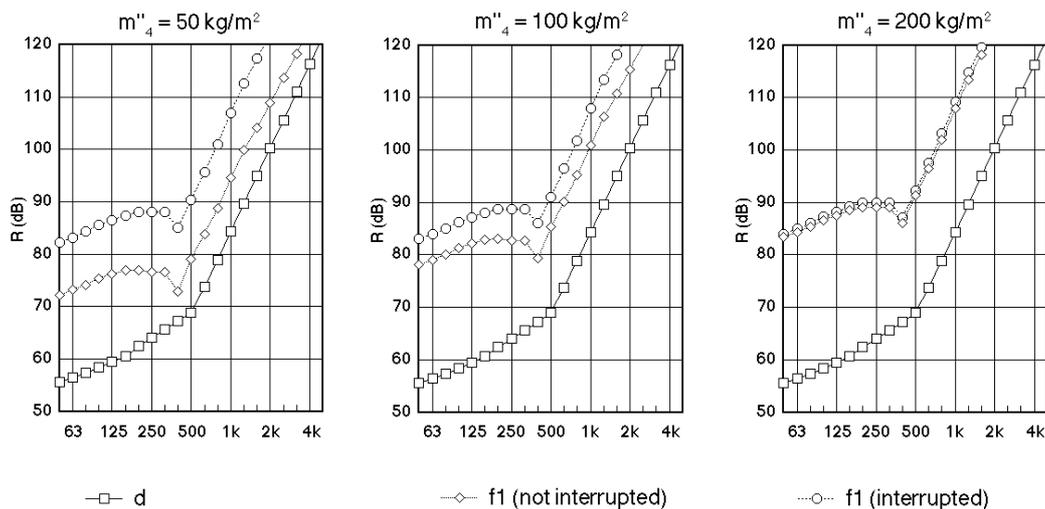
**Fig. 4:** Sound reduction index per element for different surface mass of the outer leaf (separating element:  $2 \times 100 \text{ mm}$  concrete  $2300 \text{ kg/m}^2$ , flanking element:  $100 \text{ mm}$  aerated concrete  $700 \text{ kg/m}^2$ ), without and with interruption the outer leaf with surface mass  $m''_4$ .
