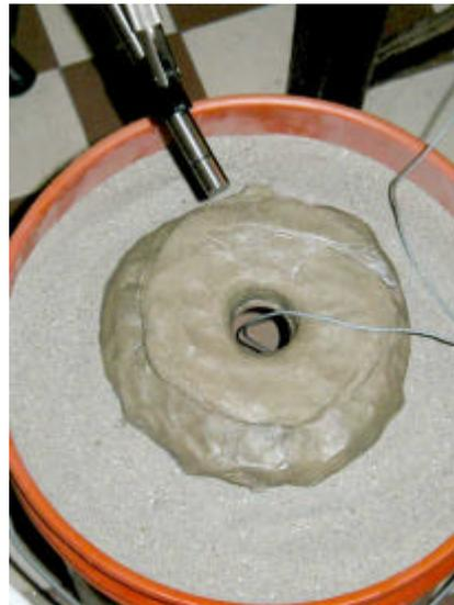
Fig. 3 - Laboratory setup for the measurement of acoustical parameters of the ceramic vessel if used as the resonator.
