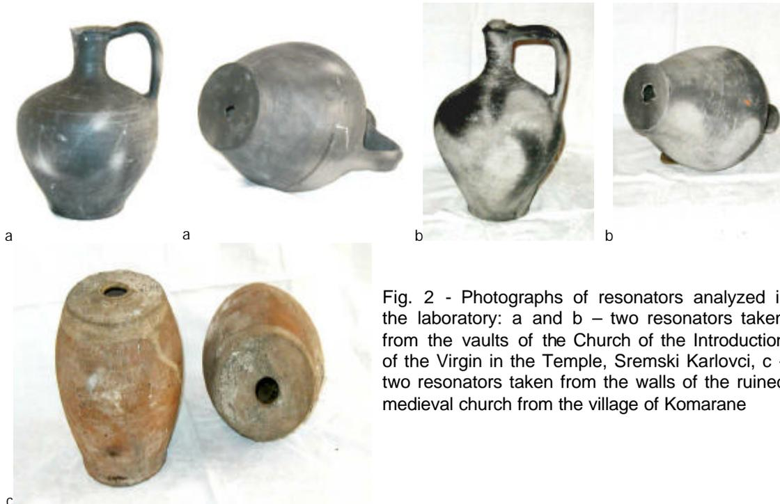
Fig. 2 - Photographs of resonators analyzed in the laboratory: a and b – two resonators taken from the vaults of the Church of the Introduction of the Virgin in the Temple, Sremski Karlovci, c – two resonators taken from the walls of the ruined medieval church from the village of Komarane
