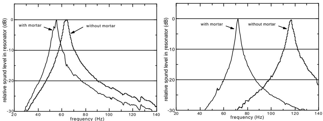
Fig. 4 - Two examples of measured resonant curves showing the mortar influence on resonant frequency: left - vessel no 1, right - vessel no 2 (all from Church of the Introduction of the Virgin in the Temple, Sremska Kamenica).
