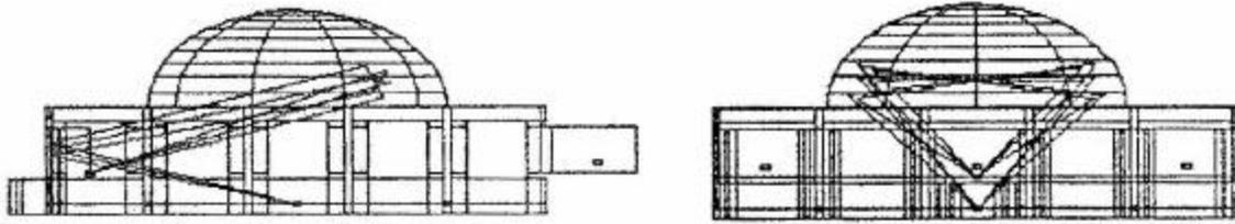
Figure 5. Ray tracing diagram of several rays forming sound concentration for ceiling shape (b).
