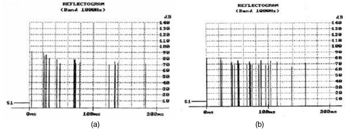
Figure 3. Reflectogram, without (a) and with (b) reflected rays potential of producing echo
