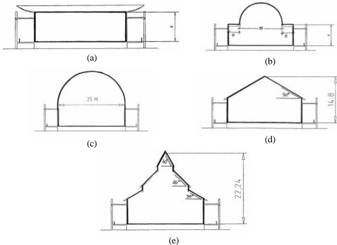
Figure 1. Section of the five ceiling shape
