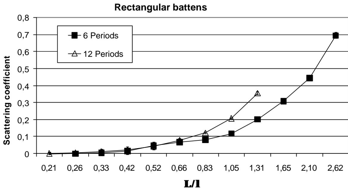
**Figure 3.** Scattering coefficients from surfaces constructed with rectangular battens in two different scales.
