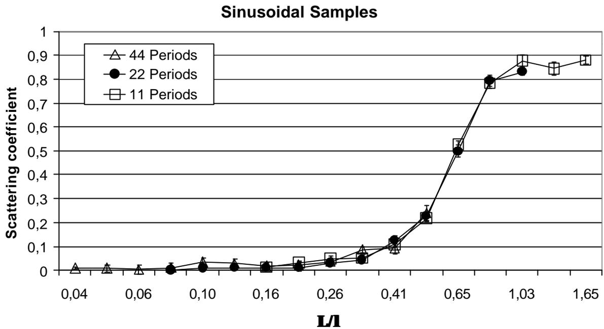
**Figure 2.** Scattering coefficients from a sinusoidal surface, constructed in three different scales.
