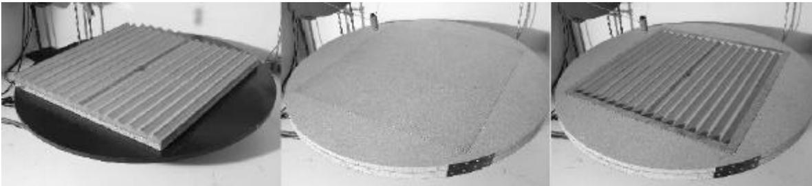
**Figure 4.** Arrangements for measuring the scattering coefficient of a square test specimen. First picture: without any correction. Second and third pictures: with correction.
