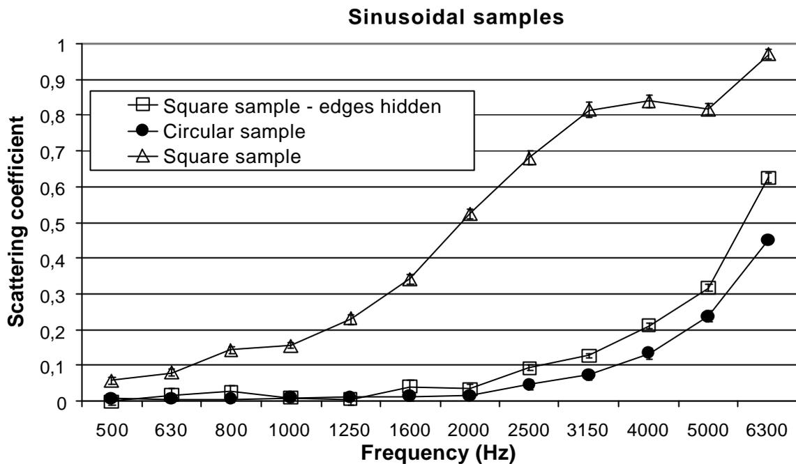
**Figure 5.** Scattering coefficients of a sinusoidal surface, measured with a circular and a square test specimen (edges hidden and not hidden).
