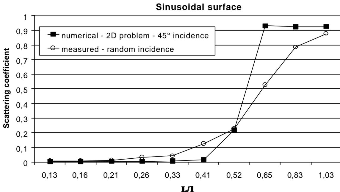
**Figure 6.** Comparison of the measured and simulated scattering coefficient of a sinusoidal surface. The simulated results were obtained from a solution of a 2D problem and for 45° sound incidence. Here  $\Lambda$  is 0,1775m (for 1000 Hz,  $\Lambda/\lambda = 0,52$ ).
