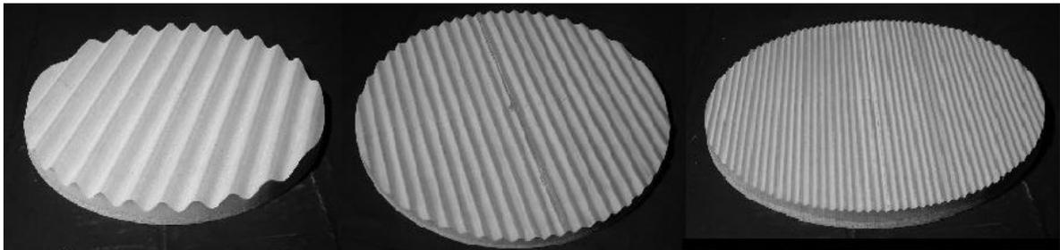
**Figure 1.** Samples of a sinusoidal surface scaled with three different factors, in order to contain 11, 22 and 44 periods.
