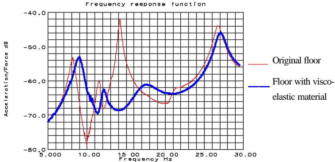
Figure 4. Comparison between measured FRF of the original floor and the floor equipped with the visco-elastic damper. The curves are average values from 11 measured points each.
