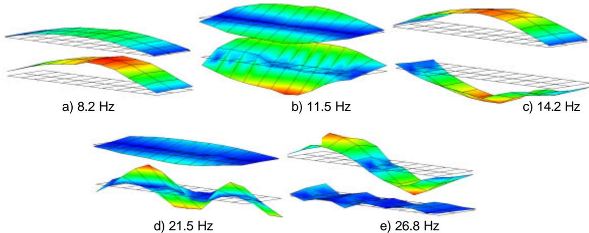
Figure 2: Mode shapes as a result of measured FRF's in 66 points. The accelerometers are equally distributed on floor (upper) and ceiling (lower).
