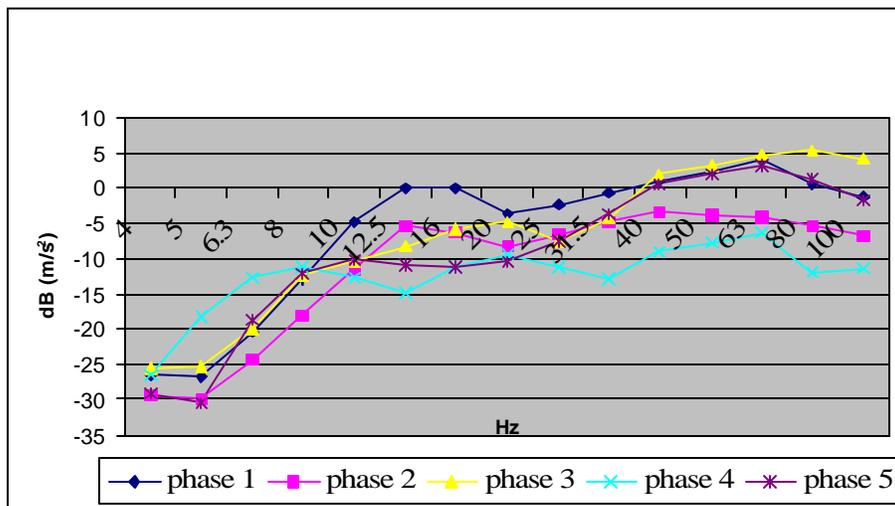
Figure 6. Acceleration plots of walking induced vibrations for different construction phases.
