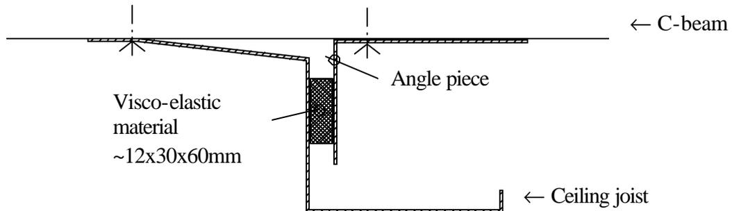
Figure 3: The visco-elastic material is mounted between an angle piece fastened to the main beam and the ceiling joist. The damping device is applied for a patent.
