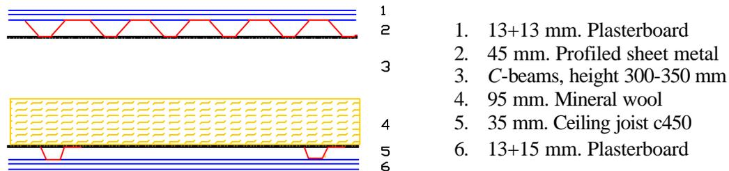
Figure 1: Design of the examined floor. The prefabricated elements have a width of 1.20m.
