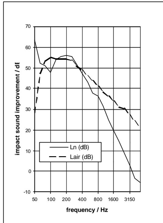
Figure 7. Airborne sound pressure level of the tapping machine in the room below the tested floor, compared with the normalised impact sound pressure level (parquet on basic structure No.4 - see table 1)
