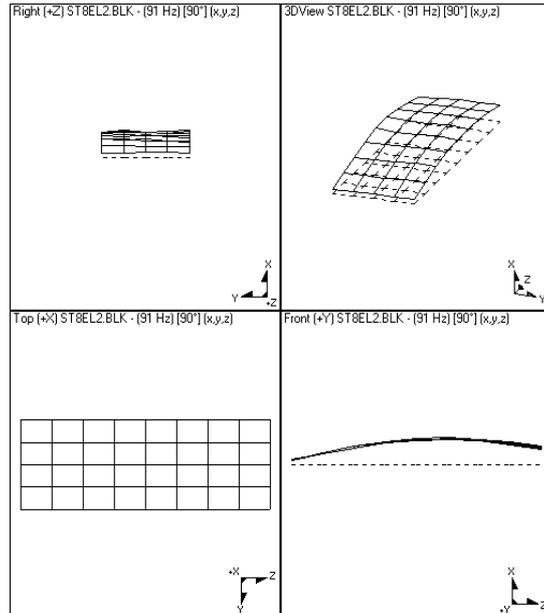
**Figure 9:** Vibration of the step at 91 Hz
