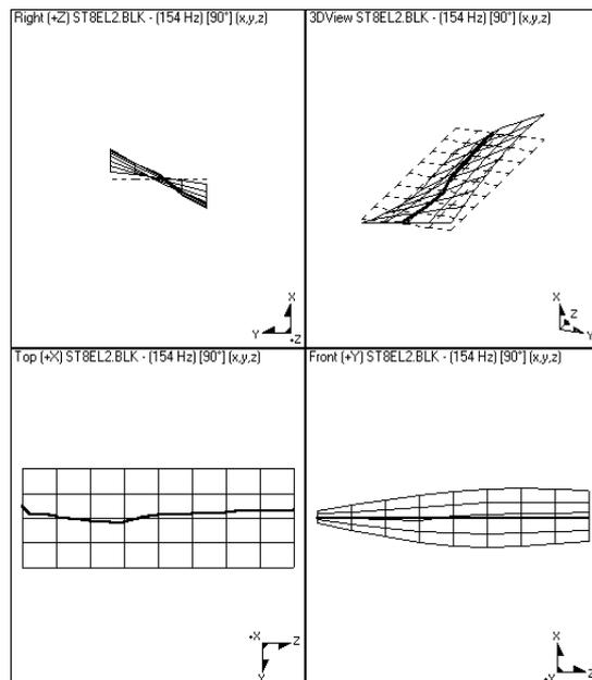
**Figure 10:** Vibration of the step at 154 Hz
