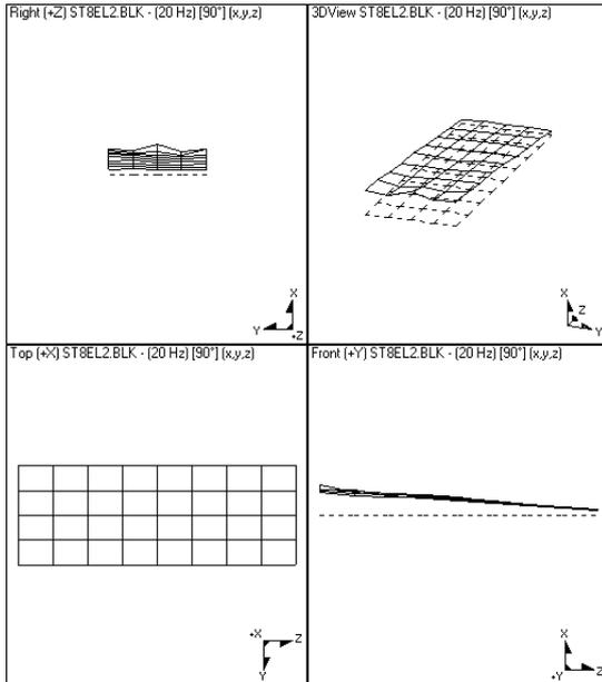
**Figure 8:** Vibration of the stair at 20 Hz
