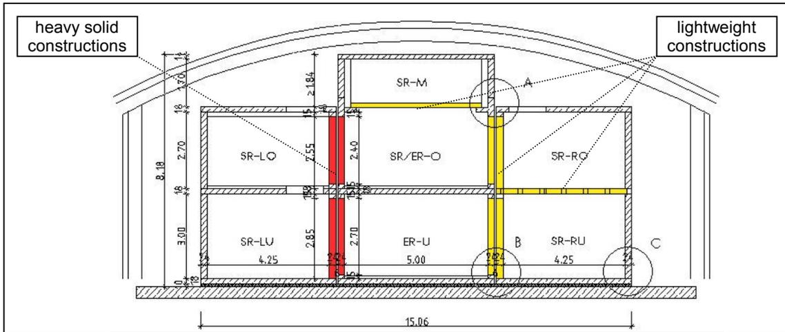
**Figure 1:** Sectional view of the new test facility for stairs
