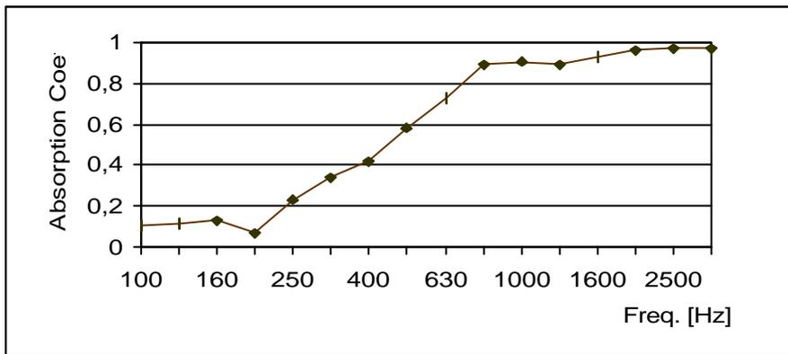
Fig. 5 – Absorption coefficients of the rockwool.
