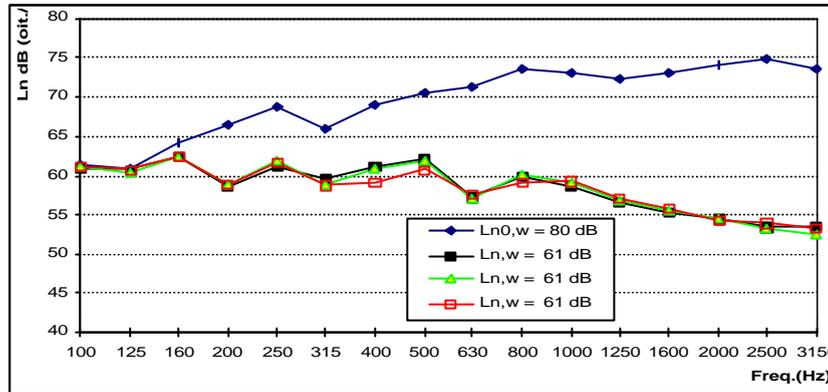
Fig. 2 - Impact sound insulation of each false ceiling
