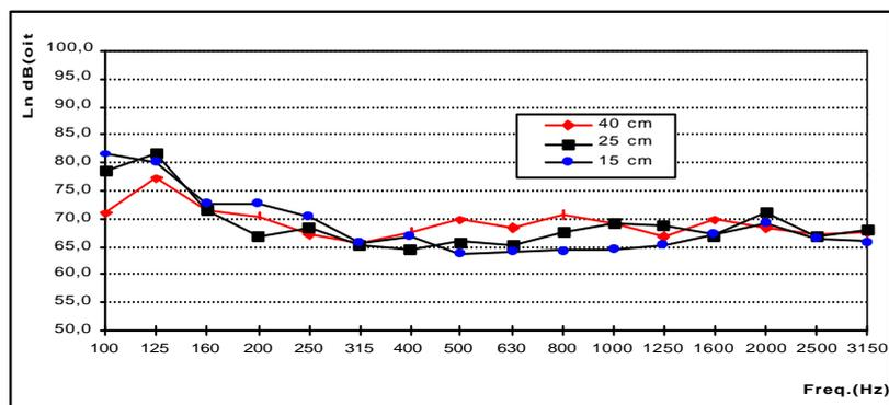
Fig. 4 - Sound field distribution inside the false ceiling cavity
