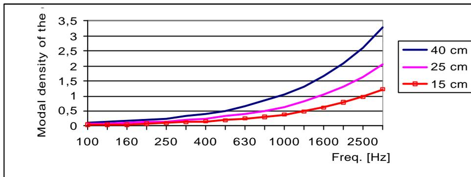
Fig. 6 - Modal density of the cavity defined by the false ceiling and the slab
