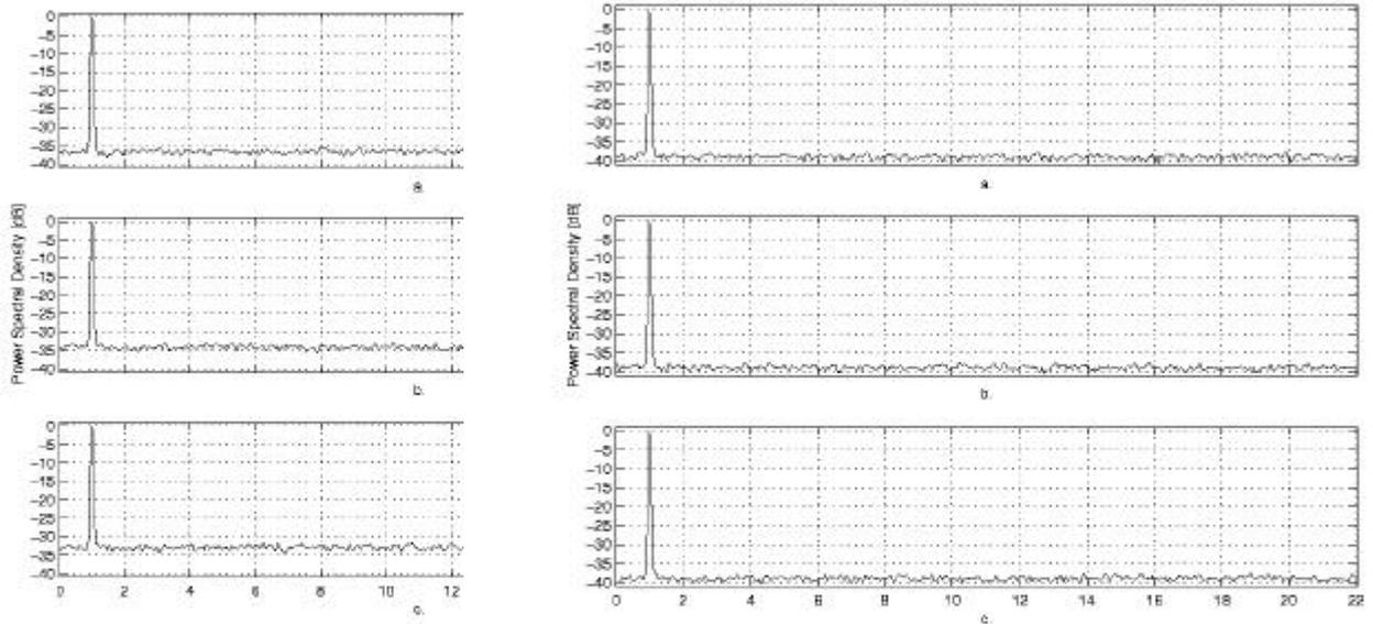
Figure 3 (Left). Power Spectral Density for a quantised 4 LSB sinusoid, nonsubtractively dithered. The PSD is normalised to give 0 dB at the input frequency. (a) 1 LSB rectangular PDF dither. (b) 2 LSB triangular PDF dither. (c)  $\frac{1}{4}$  LSB RMS Gaussian PDF dither.
