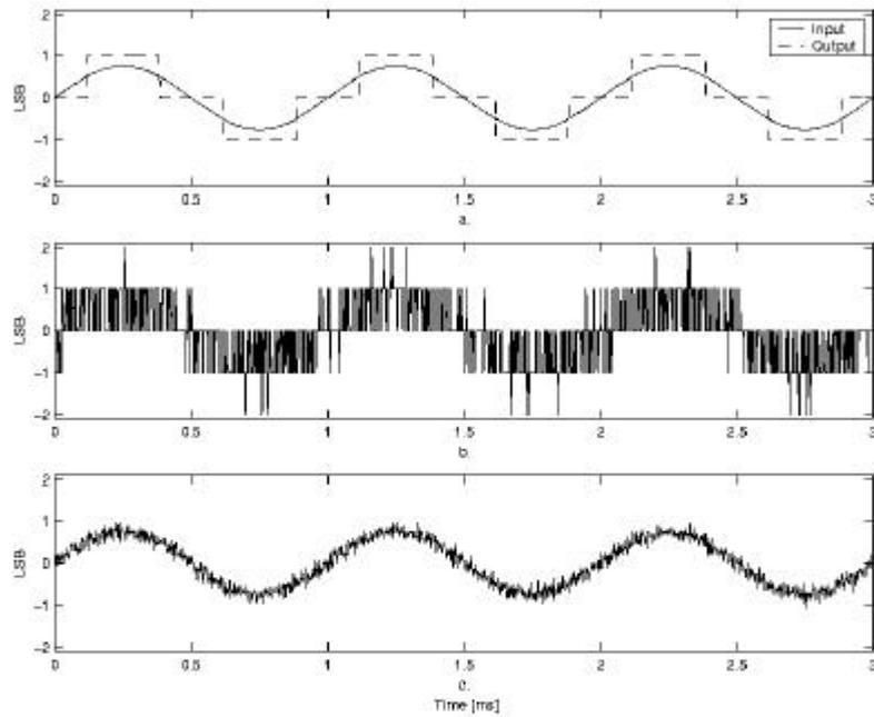
Figure 1. Undithered and dithered quantisation of  $1/2$  LSB sinusoid. (a) Input and output of an undithered quantiser. (b) Output of quantiser with a  $1/2$  LSB dithered sinusoid as input. Dithered with 2 LSB triangular PDF dither. (c) Averaged Output of quantiser. Averaged over 20 traces.
