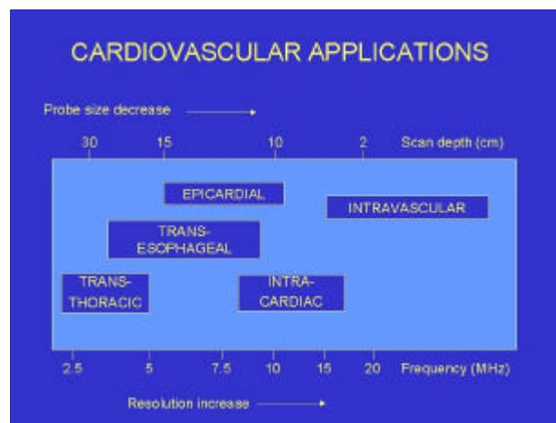
Fig. 1 - Range of cardiovascular applications with optimal frequency.
