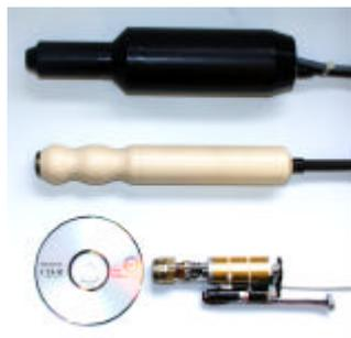
Fig. 3 - Fast rotating ultrasound probes for 3D acquisition.
