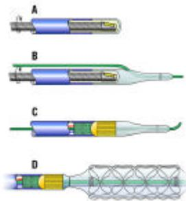
Fig. 5 - Schematic drawing of present intravascular echo catheters. Flex-shaft mechanically rotated element method (A), with guide wire (B), electronic beam switching (C) and a combination of electronic switching with a therapeutic stent placing technique (D).
