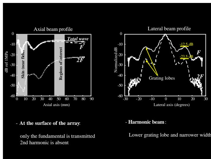
Fig. 2 - Harmonic imaging decreases transducer near field reverberation as illustrated to the left. The harmonic beam pattern has a lower grating lobe and narrower main lobe thus reducing image artefacts (figure to the right). (Courtesy A. Bouakaz)
