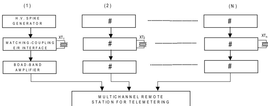
Figure 1. Schematic blocks diagram of ultrasonic stages in the remote unit.
