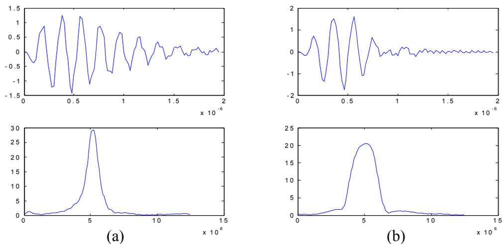
Figure 2. Computed pulse-echo responses for two combinations in the damping / inductance values. a) [120  $\Omega$ / 220  $\mu$ H] and b) [100  $\Omega$ / 22  $\mu$ H]. Pulse amplitudes are in volts, times in seconds, and frequencies in Hz.
