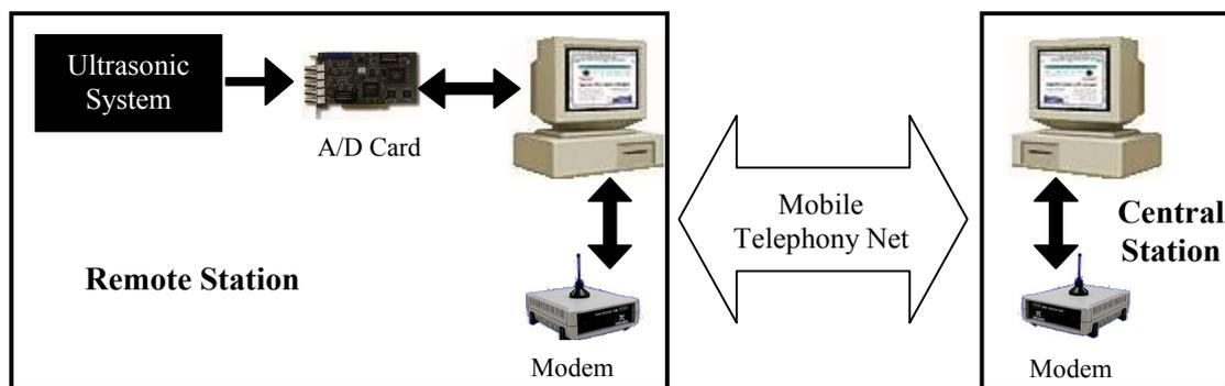
Figure 3. Laboratory prototype for ultrasonic telemetering.
