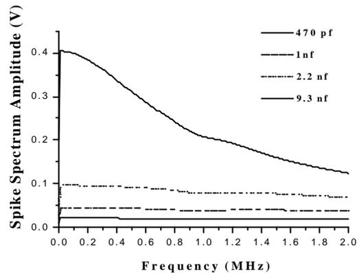
6. Spike frequency spectra amplitudes for different values of  $C_d$  and strong damping conditions ( $R_d = 22 \text{ Ohm}$ )
