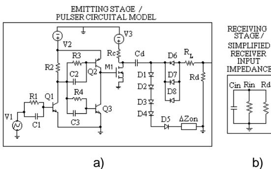
Figure 1. Emitting and Receiving models in PSPICE diagram for the electrical stages
