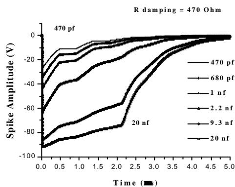
Figure 3. Driving temporal responses for different Cd values and under light damping conditions (Rd = 470 Ohm).
