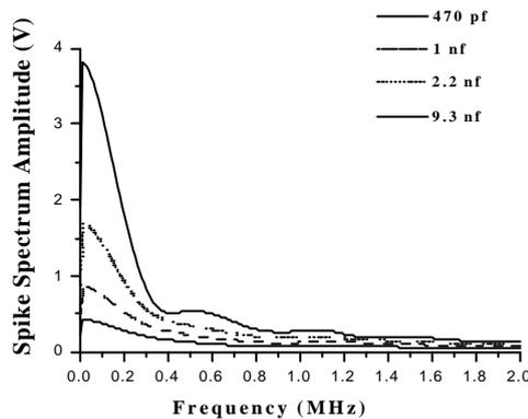
Figure 5. Spike frequency spectra amplitudes for different values of  $C_d$  and light damping conditions ( $R_d = 470 \text{ Ohm}$ ). Figure
