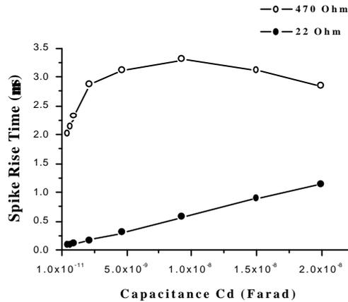
Figure 9. Behavior of the Spike Rise-Time as a function of the parameter Cd and for two different damping conditions: - light pulser damping, ● - strong pulser damping
