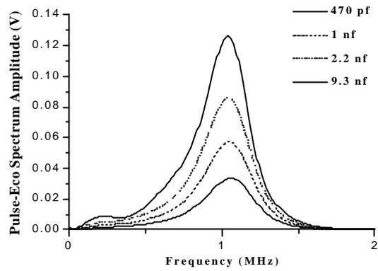
Figure 8. Pulse-Echo frequency spectrum amplitudes for different Cd values and light damping conditions ( $R_d = 470 \text{ Ohm}$ ).
