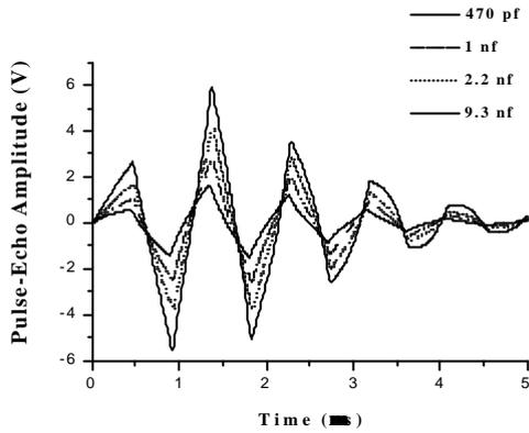
Figure 7. Pulse-Echo temporal responses for different Cd values and light damping conditions ( $R_d = 470 \text{ Ohm}$ ).
