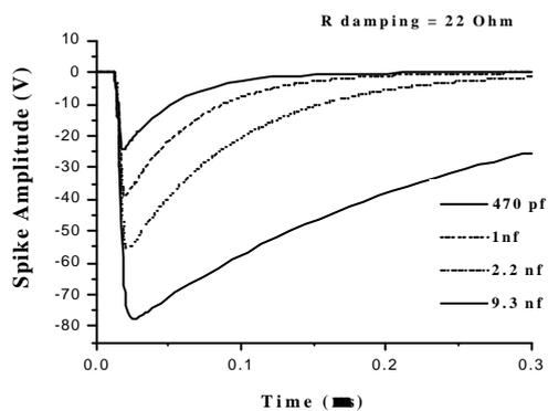
Figure 4. Driving temporal responses for different Cd values and with strong damping conditions (Rd = 22 Ohm).
