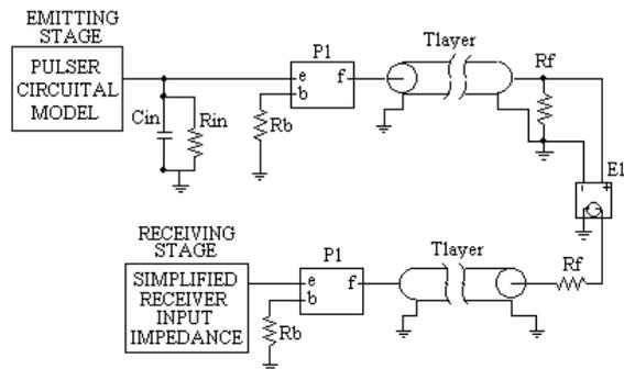
Figure 2. Pulse-echo configuration in PSPICE diagram
