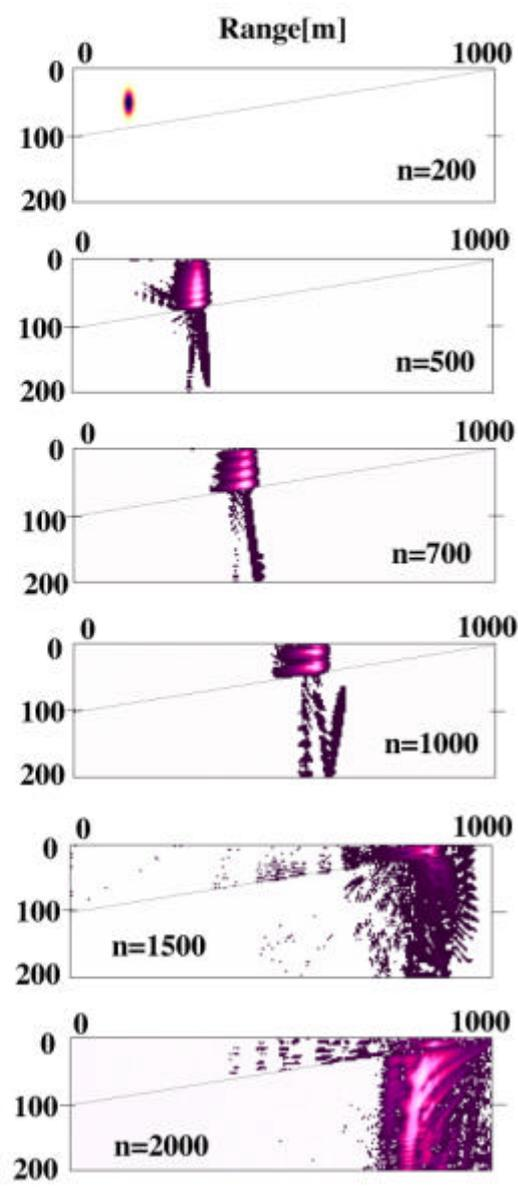
Fig.3 Pulse propagation in shallow water.
