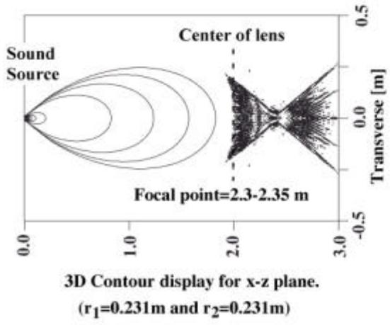
Fig.2 2D/3D model of acoustic lens and acoustical characteristics by tilt angle of incident sound source.
