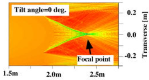
The sound source is on central axis of the lens.
