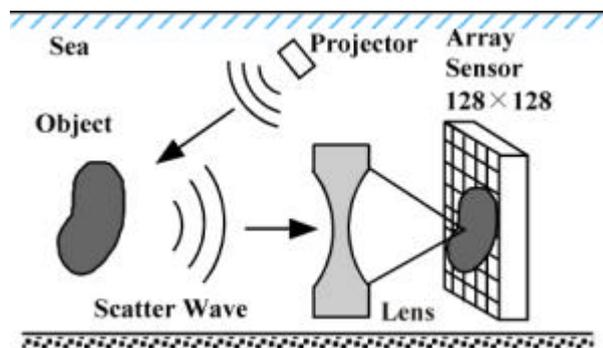
Figure 1. Real-time imaging sonar system used acoustic lens.
