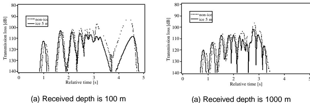
Fig. 3 Estimated receiving pulse calculated by elastic PE in Arctic Ocean.
