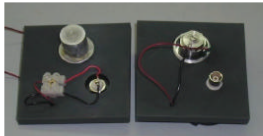
Figure 2. Two types of 36 kHz (left), and 48 kHz (right) resonant transducers inserted in the special holder
