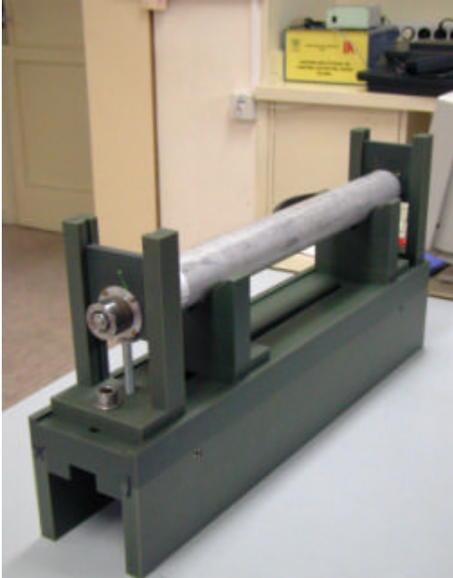
Figure 1. Support base holding an aluminium sample. One of the two transducers can be viewed on the left part of the figure.
