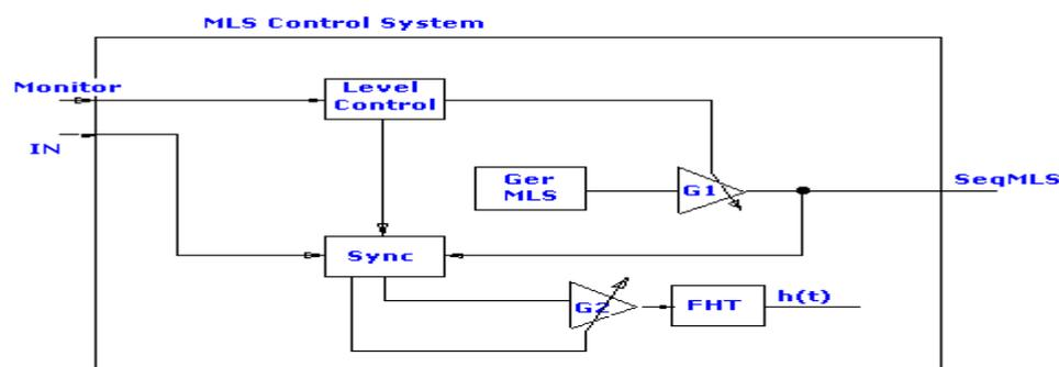
Figure 6. The basic control system for the sequence partition technique.
