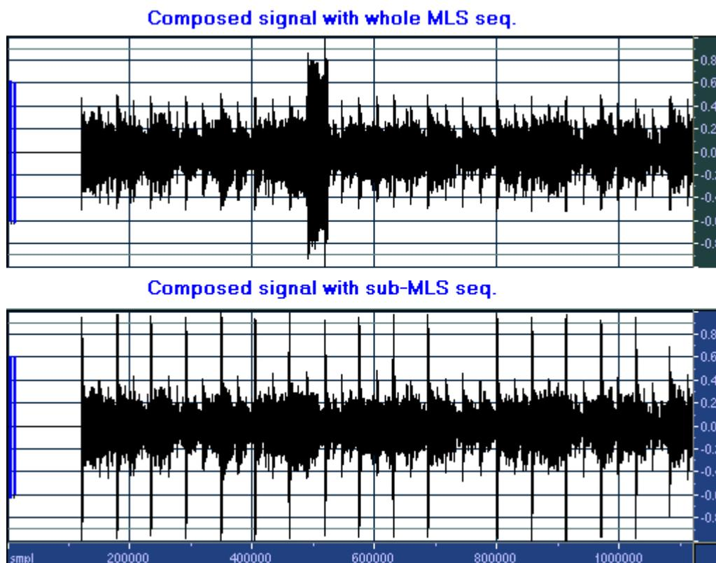
Figure 7. Input signals using MLS sequences. a) Composed Signal corresponding to a MLS sequence superimposed to a music signal track. b) Composed Signal consisting in sub-MLS sequences superimposed to a music signal track
