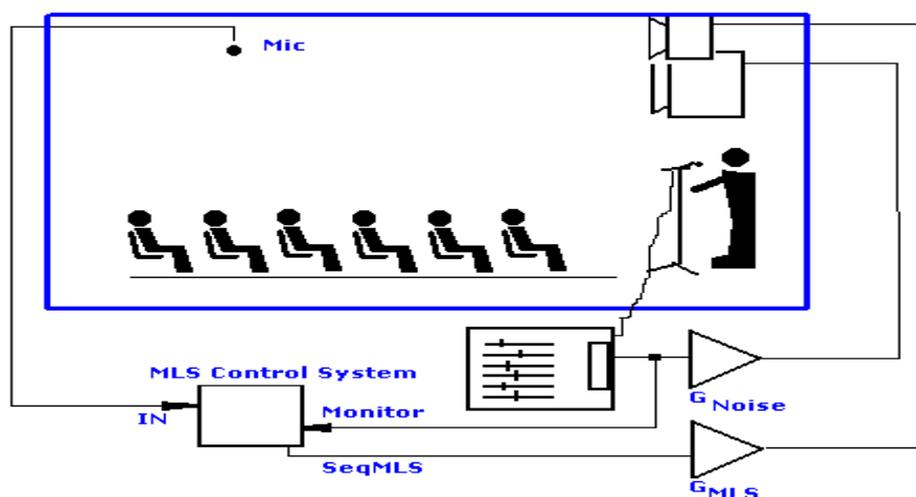
Figure 5. System lay-out for the sequence partition measurement technique.
