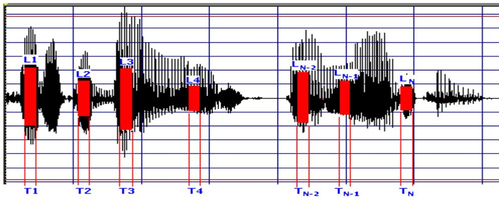
Figure 3. Implementation of the sequence partition technique, before emission.
