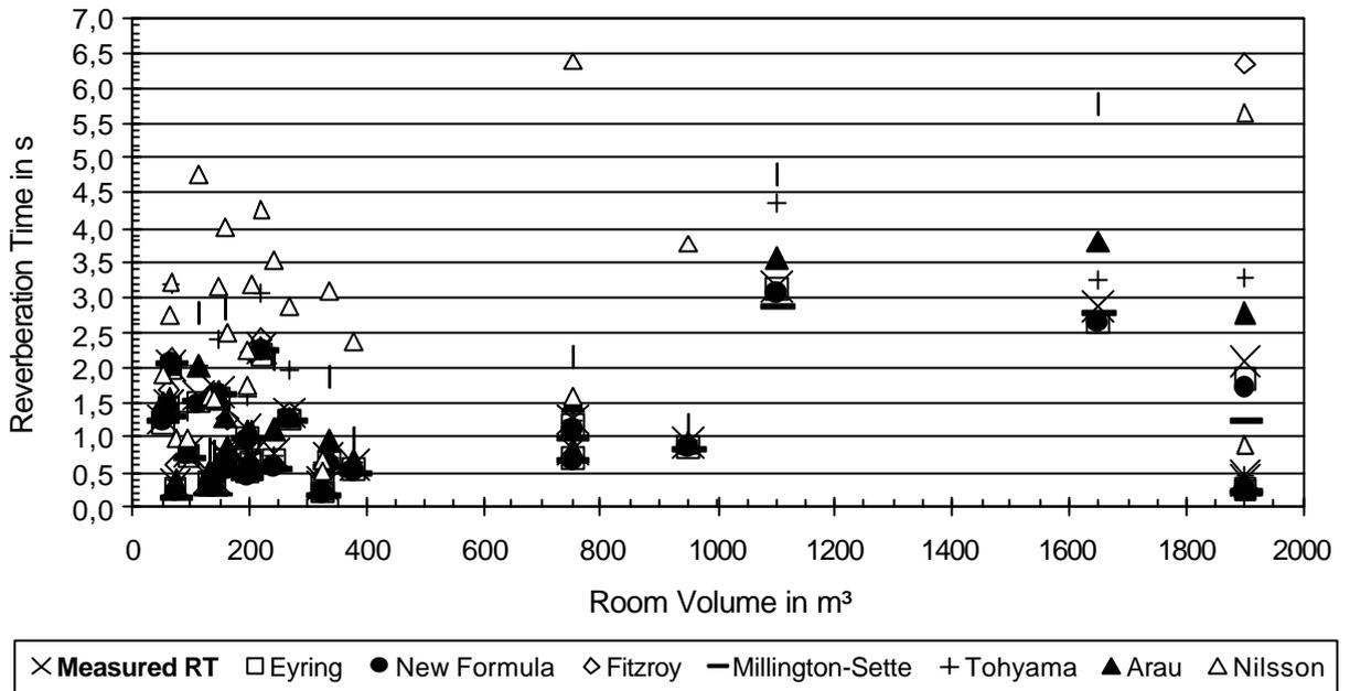
Figure 2. Calculated and measured reverberation time for different reverberation time formulae.
