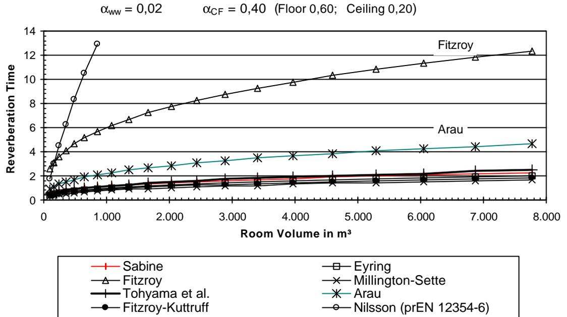
Figure 1. Calculated reverberation time for different reverberation time formulae.
