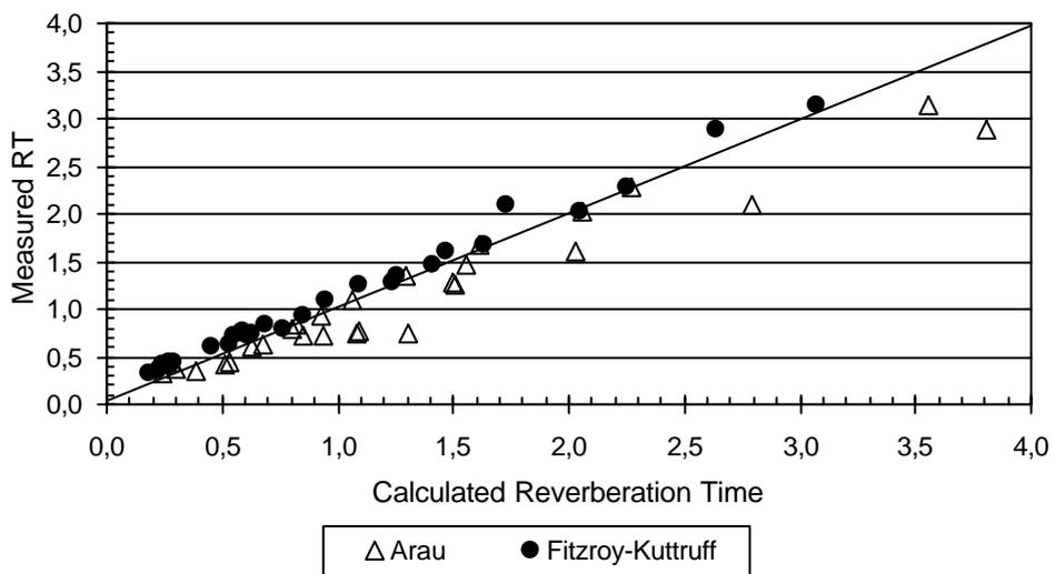
Figure 3. Comparison of calculated and measured reverberation times.
