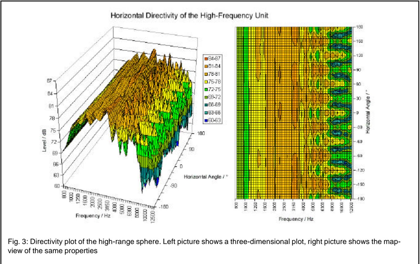
The high frequency unit which is designed as a PVC-sphere of only 10 cm diameter equipped with 12 tweeters of 1" diameter (ref. to the left picture in Fig. 1) consequently takes over at about 2500 Hz. The small cabinet was possible to realise with centre magnet drivers using neodymium with an overall diameter of only 36 cm.
