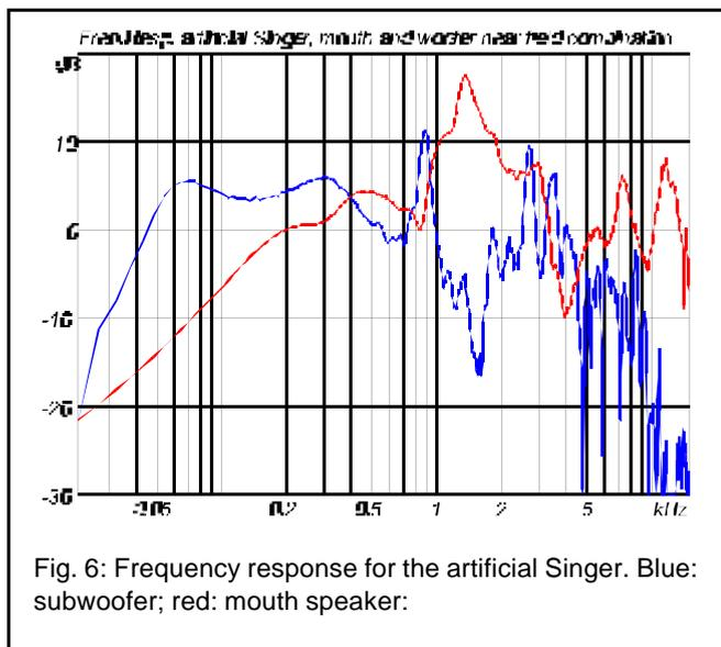
Fig. 6: Frequency response for the artificial Singer. Blue: subwoofer; red: mouth speaker:
