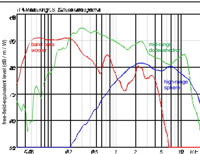
Fig. 2: Frequency response of the three loudspeaker systems. Mid- and high-range unit measured in the reverberation chamber and compensated for the absorption losses. Woofer measured in free field.
