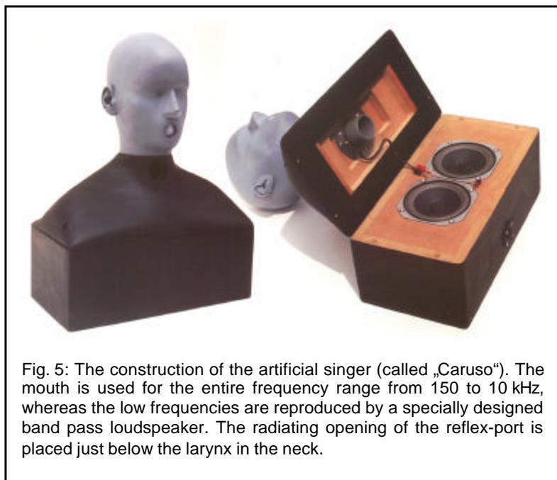
Fig. 5: The construction of the artificial singer (called „Caruso“). The mouth is used for the entire frequency range from 150 to 10 kHz, whereas the low frequencies are reproduced by a specially designed band pass loudspeaker. The radiating opening of the reflex-port is placed just below the larynx in the neck.
