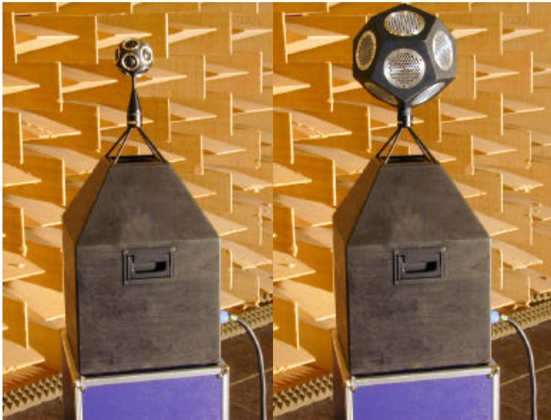
Fig. 1: Three-way measuring loudspeaker with omni-directional radiation characteristics. Note that the mid- and high-frequency loudspeakers are placed at the same centre position above the radiating vent of the woofer cabinet. They have to be replaced during measurements, which is easily handled due to the used Speakon connection
