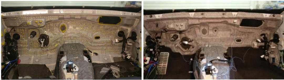
Figure 2: Firewall without insulation pad (left) and the firewall with the dash insulation pad installed (right).
