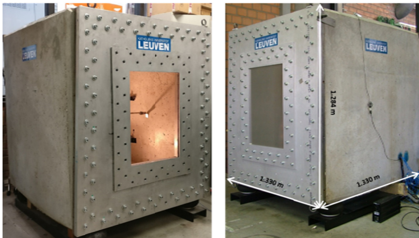
Figure 4: IL is calculated with the sound power radiated in the KU Leuven Soundbox open (left) and closed by the test sample (right) when excited by a loudspeaker.
