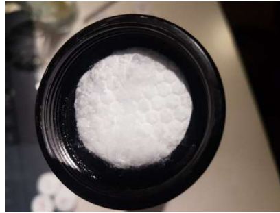
Figure 2 Sample holder testing of insulation mat
