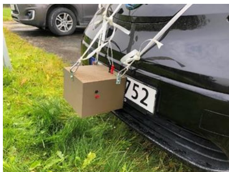
Figure 7. Mounting of loudspeaker with modified AVAS signal
