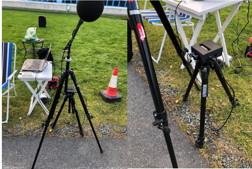
Figure 3. Microphone and loudspeaker (to the left – behind on the grass) and Lidar
