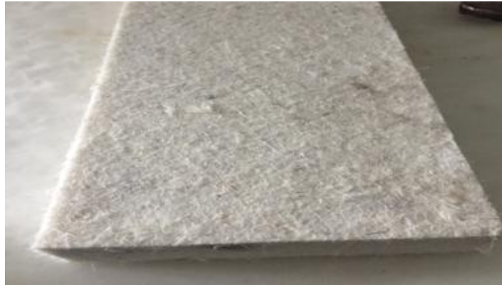
Figure 2. An example of an air-laid non woven feather mat
