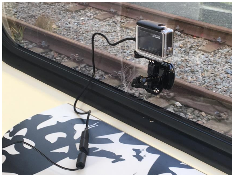
Figure 1 Recording of the exterior view using GoPro cameras attached to the window.
