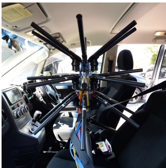
Fig. 5: Hedgehog microphone in a car cabin
