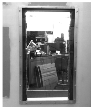
Figure 4. Dual-vented window in the 100 mm ventilation opening configuration and absorptive material fixed to vertical surfaces of the window frame
