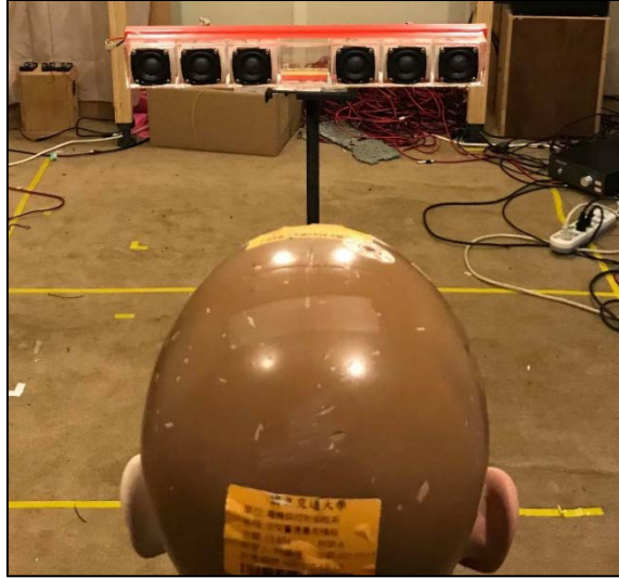
Fig. 4. Experimental arrangement of the binaural audio rendering system.
