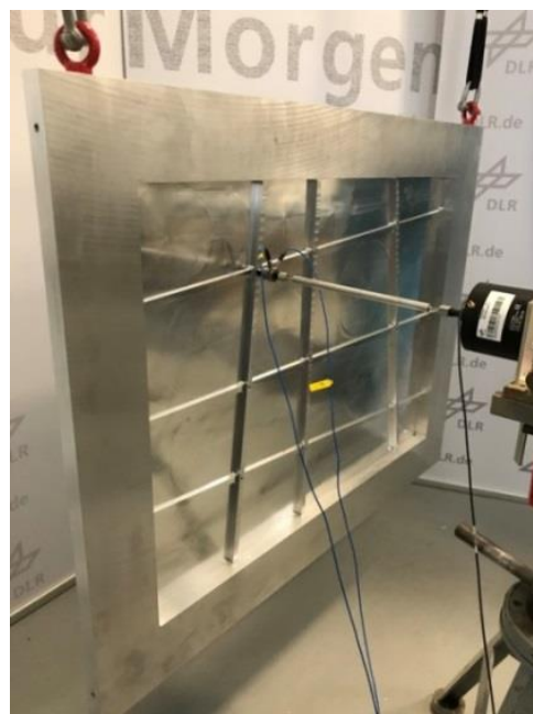
Figure 8: Aluminum plate used as test structure in a SISO configuration.
