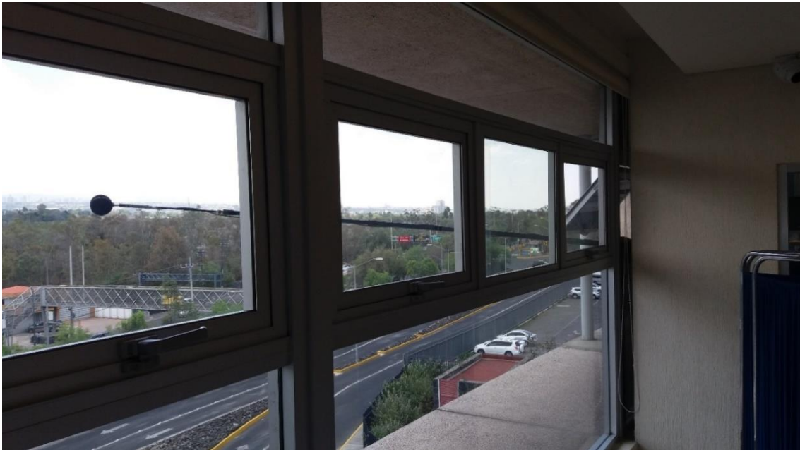
Figure 3. Position of the microphone for measuring the SPL of vehicular noise outside the classroom, 2 m front of the façade.
