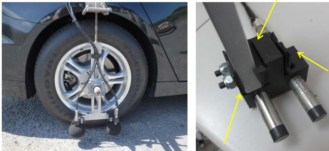
Figure 2: Modified OBSI fixture mounted on test vehicle (left) and added vibration isolation added to the probe/microphone holder (right)
