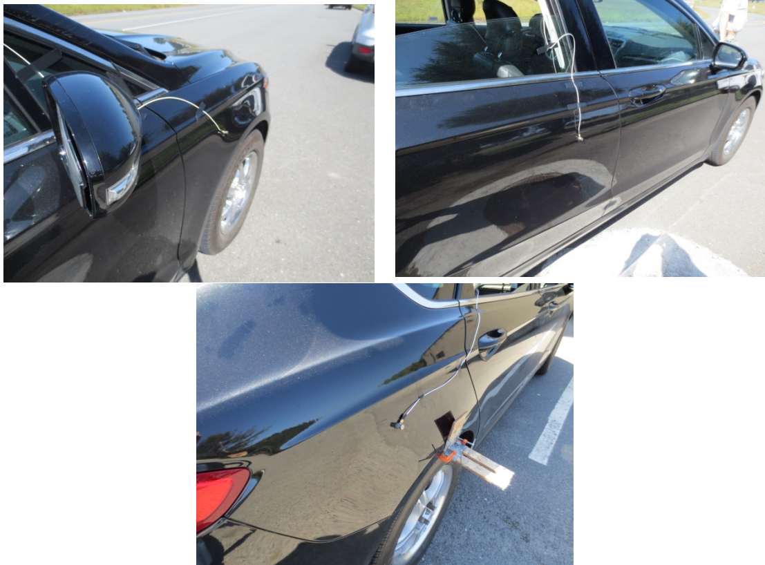
Figure 3: Body panel acceleration measurement point: front fender (upper left), rear door (upper right), and rear fender (lower center)
