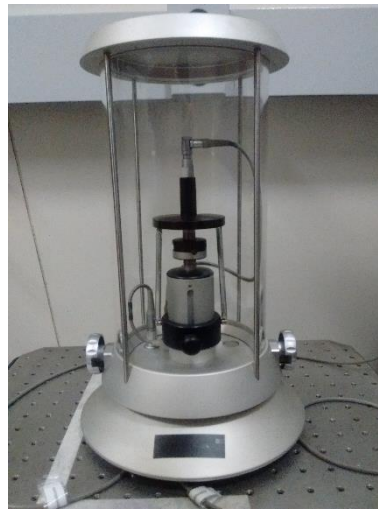
Figure 3. Microphones mounted in a plane-wave coupler.
