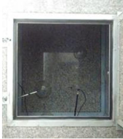
Figure 2. Reverberation chamber with microphones placed inside.
