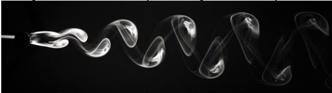
Figure 1: Vortex transfer diagram at the rear of a cylinder around a flow
