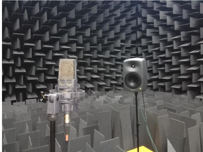
Figure 2. Free-field measurements of the AKG C414 B XLII
