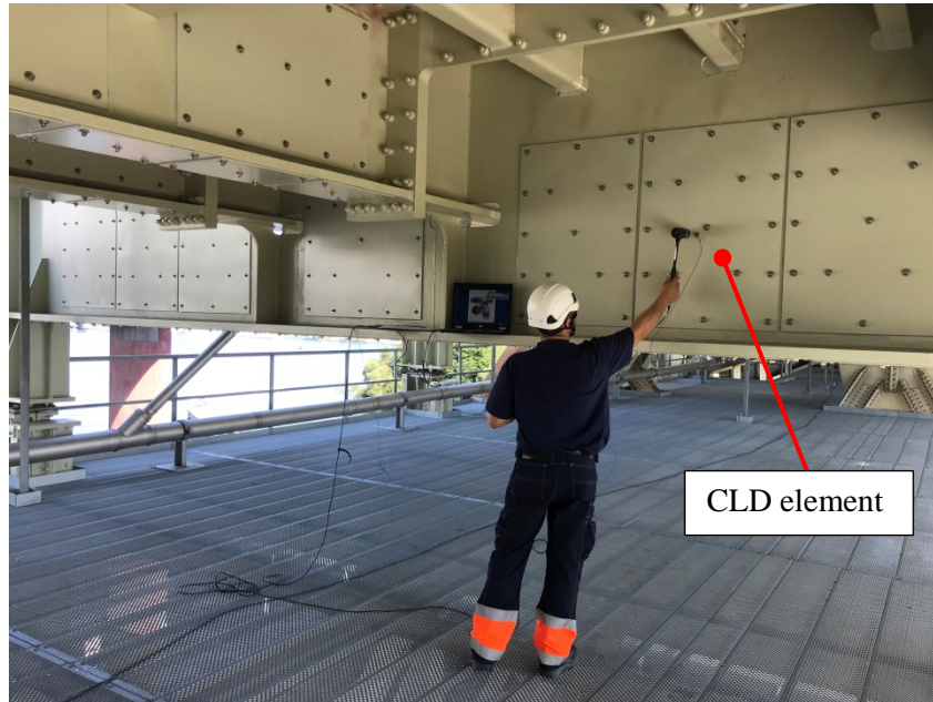
Figure 4. Point mobility measurement of transversal plate with installed CLD solution.
