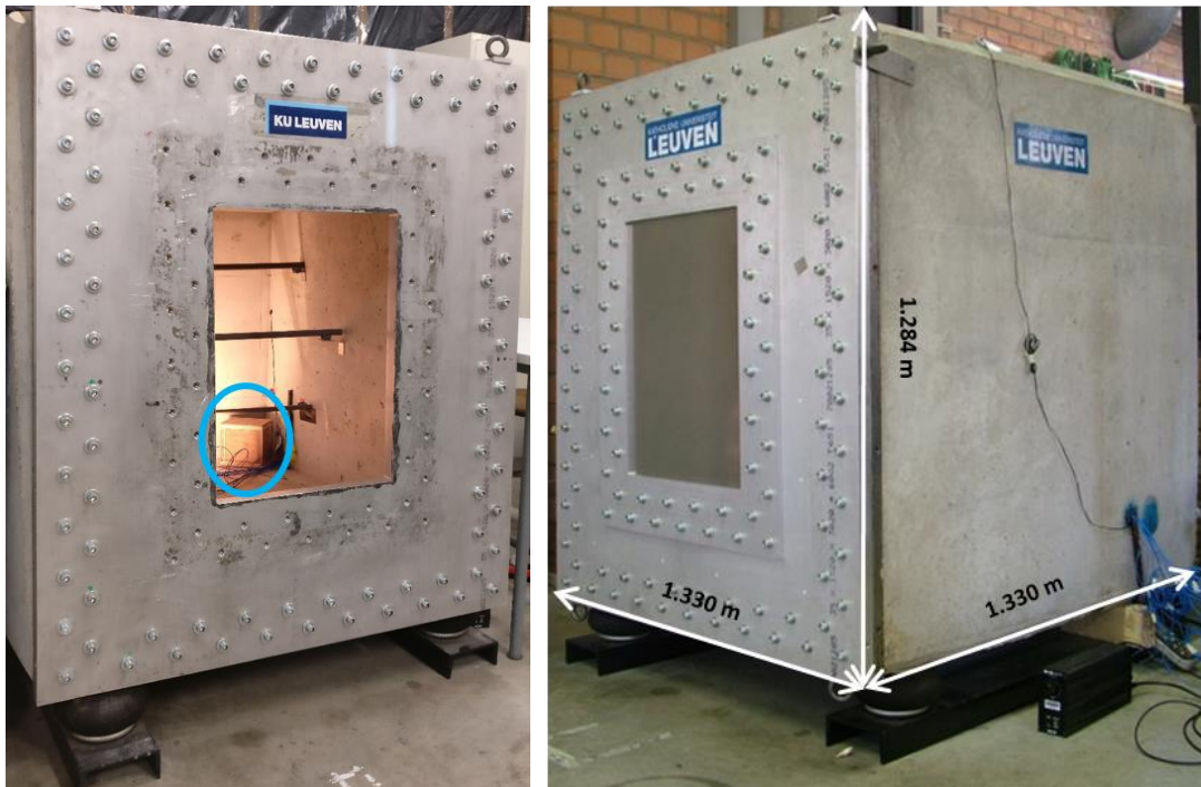
Figure 8: The sound power of the KU Leuven Soundbox aperture open (left) and closed by the tested panel (right) when a loudspeaker (blue circle) excites the cavity is measured to calculate the IL of the tested panel [10].
