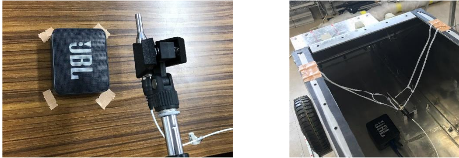
(a) Opened space (b) In cabin Fig. 6 Experimental condition for obtaining acoustic transfer function
