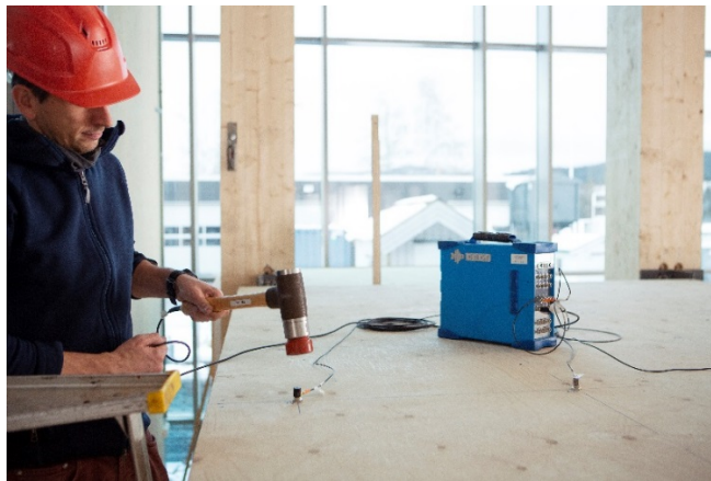
Figure 5. Illustrative picture of setup with the roving hammer technique
