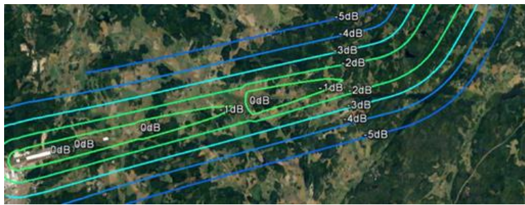
Figure 7. Comparison SAE AIR1845 and ARP866A absorption models \Delta L_{Amax, 1845-866A} dB a sample day atmosphere data over Arlanda airport
