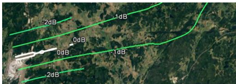
Figure 9. Comparison ISA atm and a sample day atm.as of SMHI (both modelled by ARP5534) \Delta L_{Amax, ISA-SMHI, 'spring'} dB sample day atmosphere data
