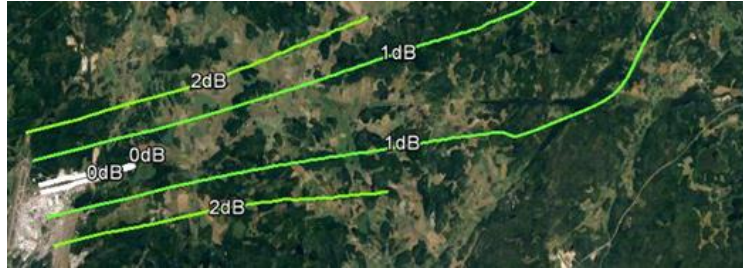
Figure 10. Comparison two sample days atmosphere data (both modelled by ARP5534 with SMHI data) \Delta L_{Amax} , 'spring' - 'summer' dB
