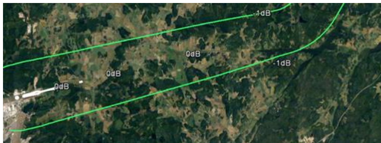
Figure 8. Comparison SAE ARP866A and the new ARP5534 absorption models \Delta L_{Amax, 866A-5534} dB sample day atmosphere data over Arlanda airport
