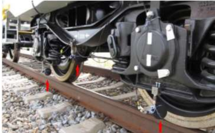
Figure 12 – Experimental set up for bogie sound source estimation
