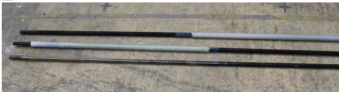
Figure 3. Drill strings used for laboratory testing: coated at the drifter end (top), coated at the bit end (middle), and a stock drill (bottom) used for baseline testing.
