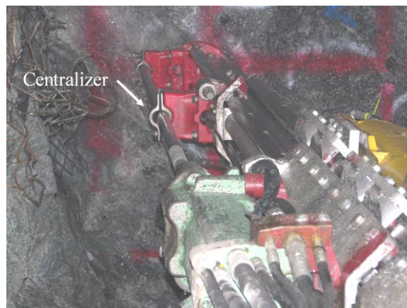
Figure 9. Location of the centralizer along the boom of the jumbo drill machine.
