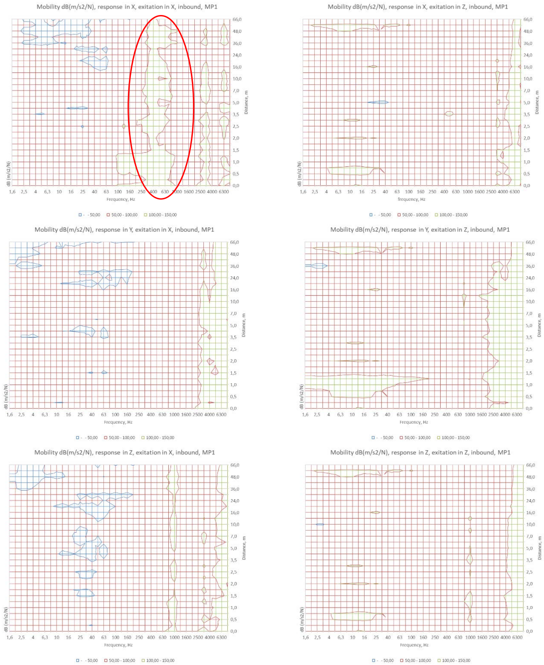
Figure 9 Mobility of the train track vs distance and frequencies. Horizontal impulse force (left), vertical impulse force (right)
