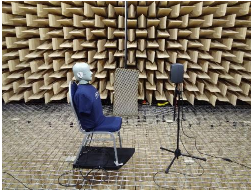
Figure 1. The artificial head in the anechoic chamber. The loudspeaker is the only source of the sound.
