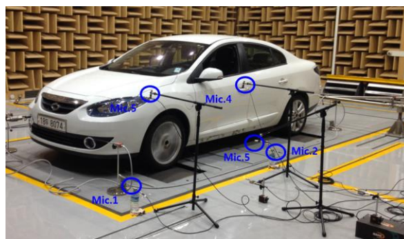
Figure 3. Indoor noise test method on dynamometer
