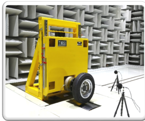
Figure 2: Drum facility showing the position of center and trailing microphones
