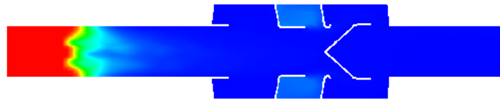
Figure 3 – Temperature distribution inside the silencer
