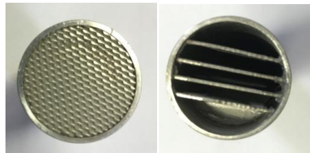
Fig. 9. Sample of MPP with designed five cavities L-type structure.
