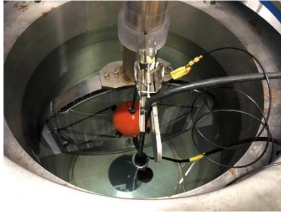
(c) The VHS90 particle velocity receiver fixed on the ring in standing wave tube
