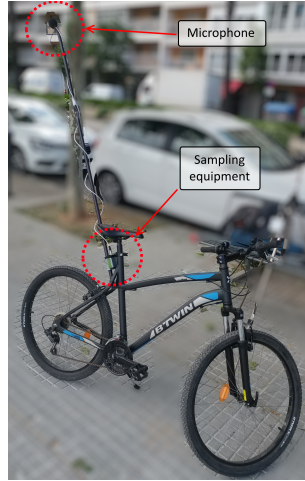
Figure 2: Bicycle with the measuring device mounted under the seat. The microphone is located at the top of a tube at an approximated height of 2 m.
